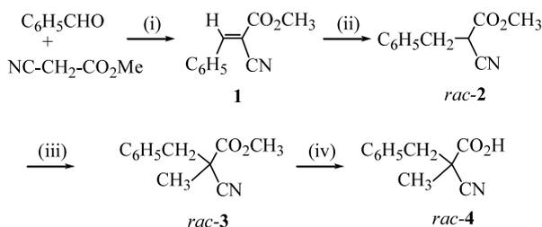
**Scheme 1.** Reagents and conditions: (i)  $\text{NH}_4\text{AcO}$ ,  $\text{AcOH}$ ; (ii)  $\text{H}_2$ ,  $\text{Pd/C}$ ,  $\text{THF}$ ; (iii)  $\text{K}_2\text{CO}_3$ ,  $\text{CH}_3\text{I}$ , acetone; (iv)  $\text{KOH}$ , methanol.
